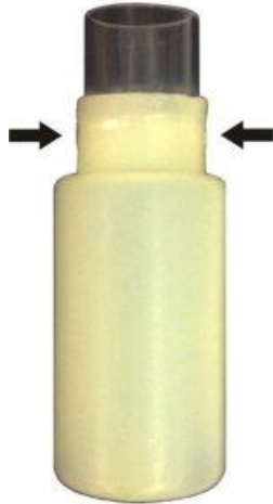
Figure 1. Plastic beaker for CFE calibration in stereotaxic frame
