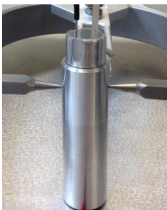
Figure 2. Beaker (Invilog micro-stirrer) fixed between ear bars
